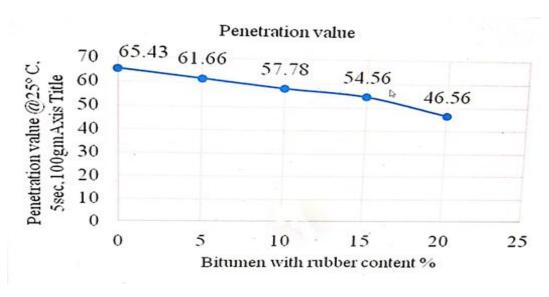
Fig. 8. Penetration value versus % of rubber waste
