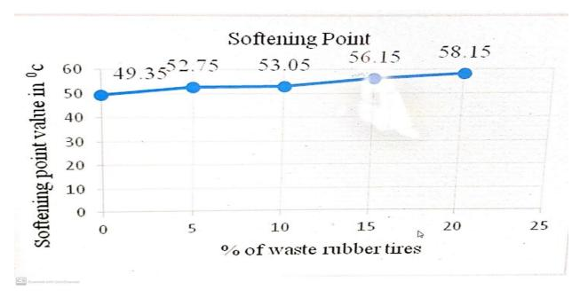
Fig. 9. Softening point Value versus % of rubber waste
