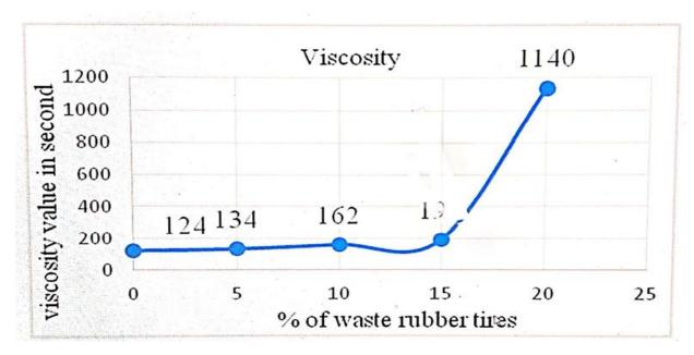
Fig. 10. Viscosity value versus % of tire rubber waste
